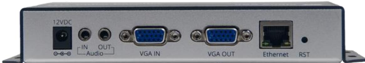
The Front-panel text gives you IN- and Loop-Output connections Audio and Video (VGA separately). Use the delivered 230VAC -> 12VDC PSU and do not use Voltage higher than that. Note: VGA does not have internal Audio like HDMI. Right: RESET Hole (internal button)= Restores factory settings by pressing 5-10 seconds
